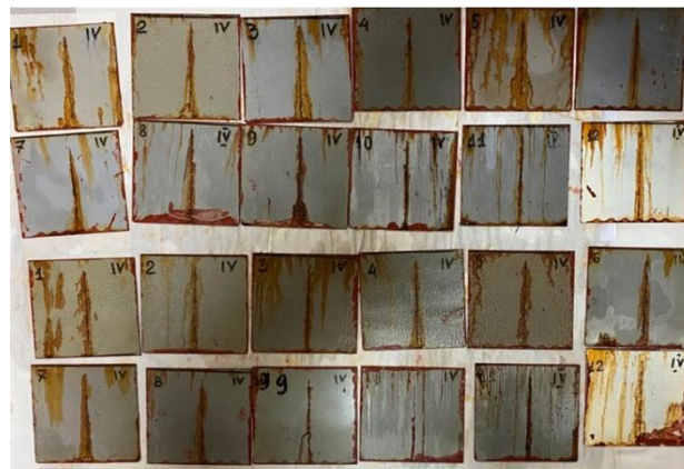
Fig. 1. Visual inspection of the test panels after 200 hours of exposure. Samples cured at 25 °C (Rows 1–2) versus post-cured at 100 °C (Rows 3–4).
